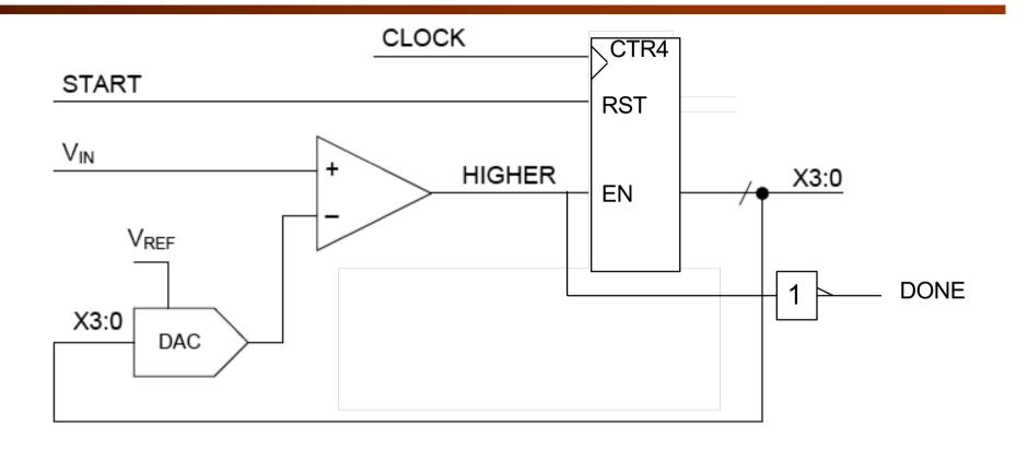
Here is a simple ADC using a DAC, a comparator and a binary up counter.
